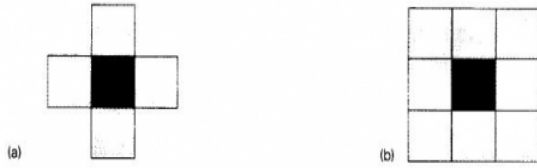
Figure 1: The first neighborhood approach is referred to as the "Five-neighbor square", or the von Neumann neighborhood. The second neighborhood is the "Nine-neighbor square." [4] The sandpile model uses the von Neumann approach.
