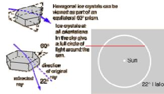
Further refinement using  $n=1.306$  for red and  $n=1.317$  for blue gives angles of  $21.54^\circ$  and  $22.37^\circ$  for red and blue respectively. The inner edge of the halo is sharp and appears redder - the angle of minimum deviation for red is less, so red is seen from crystals closer to the Sun or Moon direction (inside of ring).
